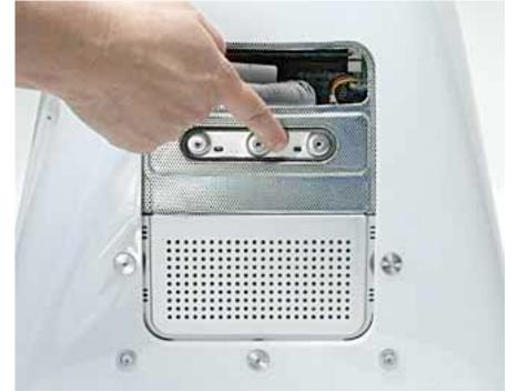
protect the computer from damage caused by electrostatic discharge. **Important:** To avoid electrostatic discharge, always ground yourself by touching metal before you touch any parts or install components inside the computer. To avoid generating static electricity, do not walk around the room until you have finished installing the memory and closed the computer.
