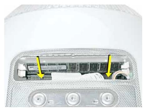
9. Push the ejectors on the memory slot outward and down so they are in the open position. The module is designed to fit into the slot only one way. Be sure to align the notches on the module with the small notches inside the slot.
